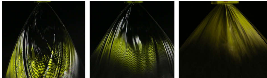
Fig. 12. Images captured with the interferometric technique. (Left) 0.5 bar, (center) 1.5 bar, (right) 3 bar.
