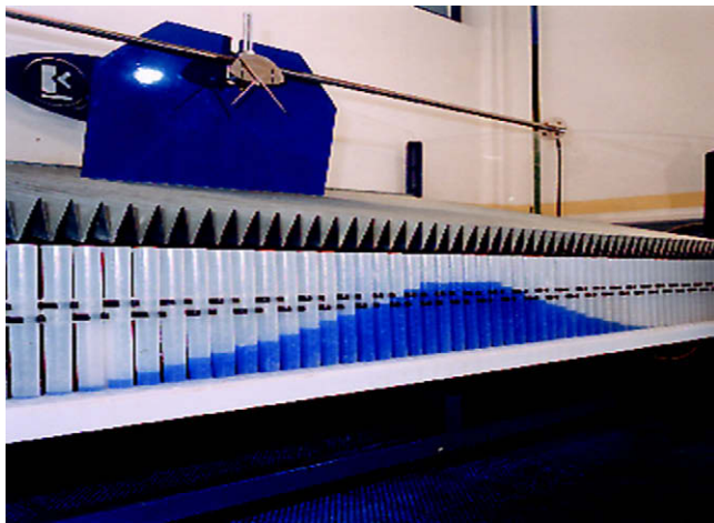
Fig. 14. Experimental device employed for flow distribution measurements (Patternator).
